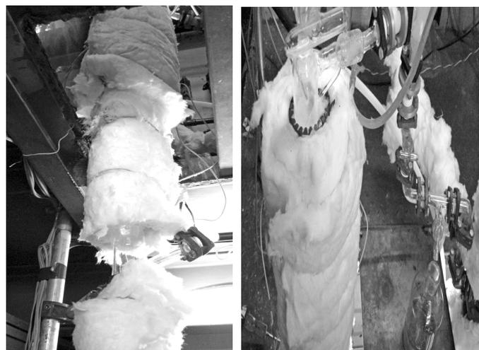
Figure 3: Sulfuric acid decomposer (left) and  $\text{SO}_3$  decomposer (right) during operation.
