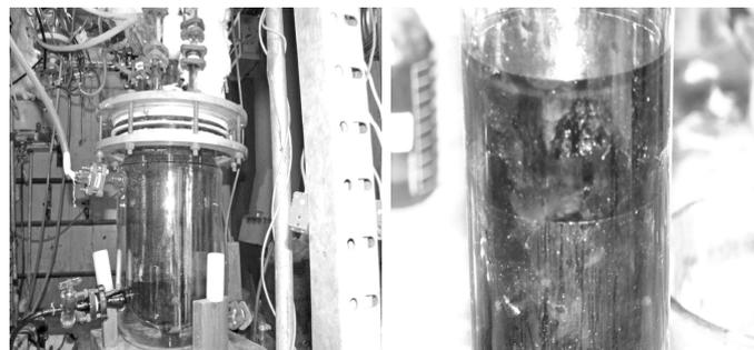
Figure 2: Bunsen Reactor of glass system and liquid liquid separator
